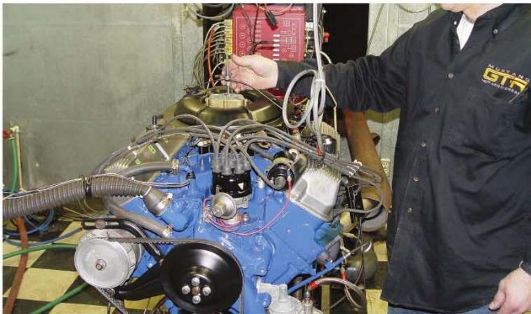
**MAX AIRFLOW:** We have a modified GM air cleaner base that we use during almost all of our dyno sessions to see if the airflow into the carb can be improved. Our Holley liked it in Test 12, netting us an additional five horsepower, although with no increase in peak torque. The average numbers tell the real story. Average hp went up by 3.6, and torque by 3.7 lb-ft for our best numbers of the day.
