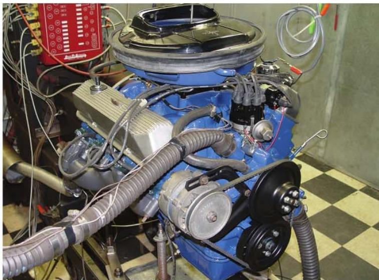
**BREATHING APPARATUS:** For the last test, we installed the complete Cougar Ram Air air cleaner assembly, including the old dirty paper air filter. We were surprised that it didn't really hurt power all that much, knocking off about seven hp and eight lb-ft of torque.
